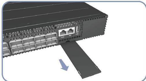
1 The switch product label is located below the Mgmt and Console ports on the right side of the front panel. Pull the label out to view the product information.
